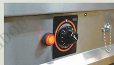
The temperature of the water-boiling pot is controlled by the thermostat that allows 10 levels of output. The right in the picture is where a high limit sensor for deep-frying or stewing is installed. It is used as an overheating prevention device.
