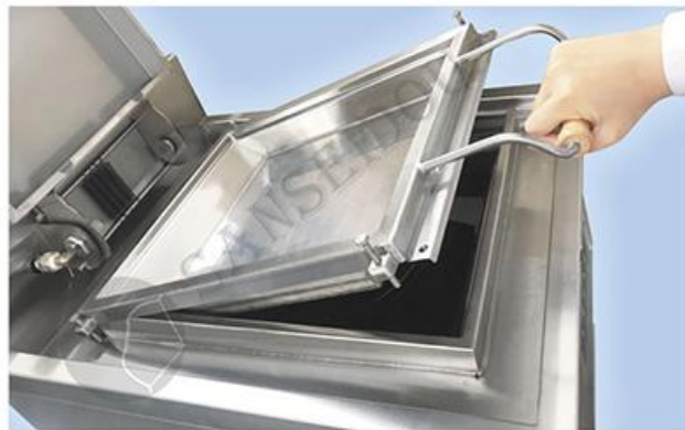
It is convenient to clean. The grill pan can be lifted, the water and the garbage can be flowed into rear trash basket.
