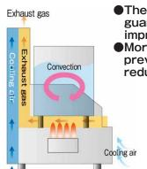
The exhaust gas exhausted along the back guard heats the back of the pot, which improves the thermal efficiency.
