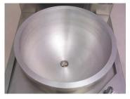
Casted-in heaters concentrated especially in the front side focus on heating up the front side of the pot, generating strong convection currents from front side toward back side. This makes noodles turn around in the pot vigorously and boil in a delicious manner.
